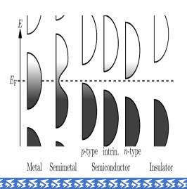
\*\*\*\*\*\*\* Filling of the electronic states in various types of materials at equilibrium. Here, height is energy while width is the density of available states for a certain energy in the material listed. The shade follows the Fermi–Dirac distribution (black: all states filled, white: no state filled). In metals and semimetals, the Fermi level EF lies inside at least one band.
